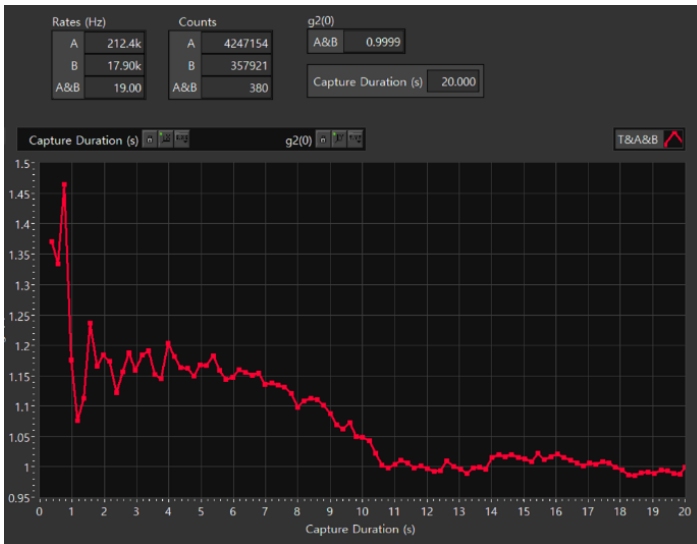
Figure 6. Representative 20 s HBT acquisition of the attenuated laser.
